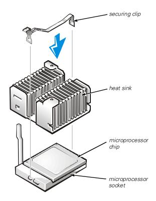
Figure 8-13. Installing the Heat Sink
